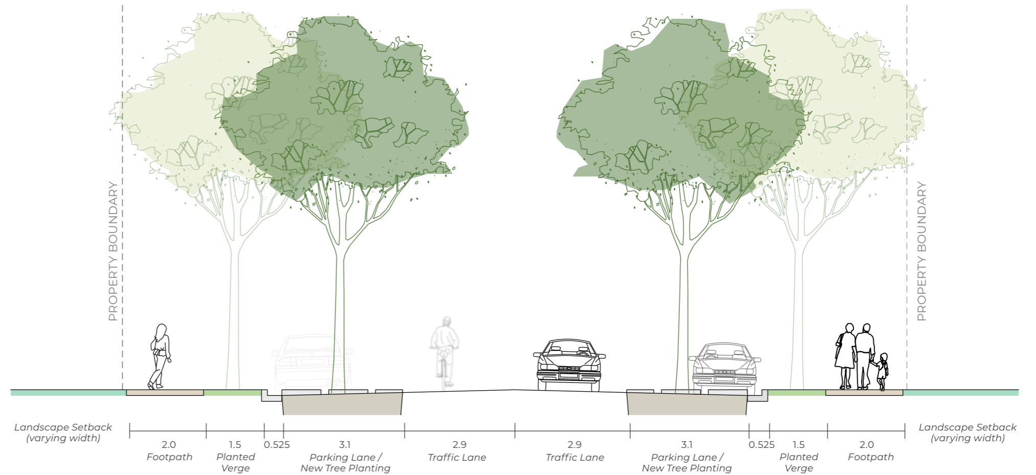
Figure 61. Section BB - Typical Section of Slow Streets. Source: CLOUSTON Associates
